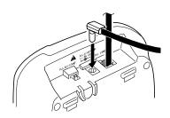
4. Route the adapter's cord through the strain relief slot on the base.
